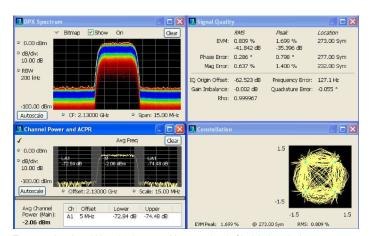
Time-correlated, multidomain views provide a new level of insight into design or operational problems not possible with conventional analysis solutions. Here, ACLR and Vector Modulation Quality (Opt. 21) are performed on a single acquisition, combined with the continuous monitoring of the DPX $^{\otimes}$  spectrum display.
